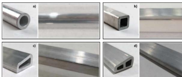
*Extrusions made from AA6063 industrial scrap by ShAPE producing (a) circular, (b) square, (c) trapezoidal, and (d) two-cell trapezoidal profiles.*
