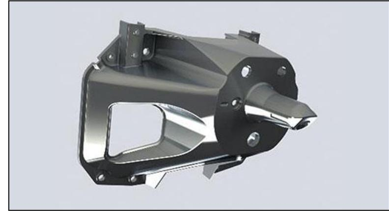
Prototype Wrangler Spare Tire Carrier
